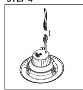
Plug the female connector of the RETROFIT KIT onto the male connector of the QUICK CONNECT ADAPTER.
