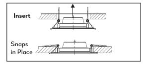
Holding spring clips against fixture, carefully insert the fixture into the hole. Continue to slide in the fixture, releasing spring clips, until clips snap into place. Ensure the fixture is flush against the ceiling and securely in place.
