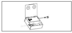
Make wiring connection inside the junction box using the EZ connectors (as shown above). Connect the 120V line wire from your house electrical to the black wire (black to black). Connect the neutral wire to the white wire (white to white).
