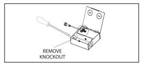
Using a screw driver, carefully remove the knock out as shown above.
