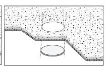
Cut a hole in the ceiling for your fixture. Before you begin, ensure that the hole you are going to be cutting does not interfere with studs, piping, electrical or other building structures. See the above chart for cutting size or refer the the appropriate template for your model.
